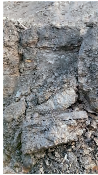
Rys. 6. Fragment skarpy po próbnym hydro-cięciu Fig. 6. A fragment of the slope after a trial hydro-cutting
