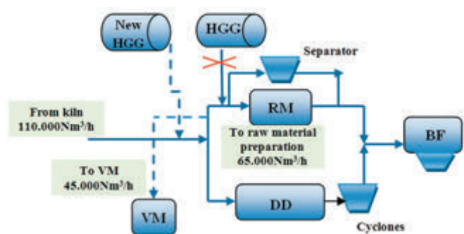
Fig. 1. Flow-chart of gasses distribution (Legend: K4-Rotary kiln; VM-Vertical Mill; HGG-Hot Gas Generator; RM-Raw Mill; DD- Drum Dryer; BF-bag filter)
