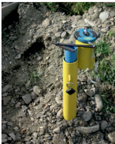
Rys. 14 Pomiar osiadań Fig. 14 The subsidence measurements
