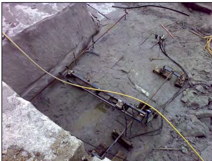
Rys. 4.33. Perforator firmy Perfora – kopalnia Skalimex (granit)
