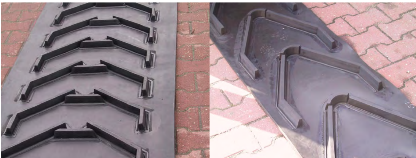
Rys. 7. Profil H-35 mm do pracy w niecce wzór 35-11 i profil H-40 mm wzór 40-09 Fig. 7. H-35 profile suitable for a trough belt conveyor, pattern 35-11, and profile H-40 mm, pattern 40-09
