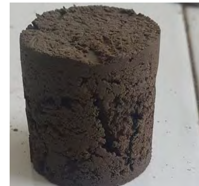
Soil from borehole S-2 collected with a bulk density ring
