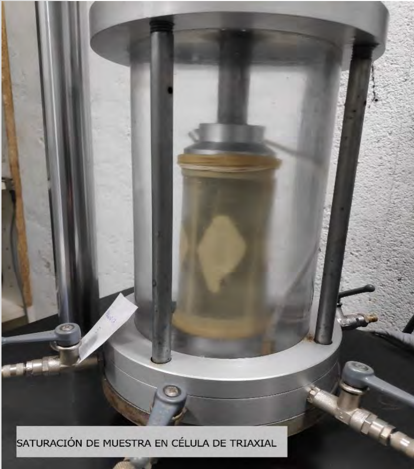
Core sample saturation process in triaxial cell
